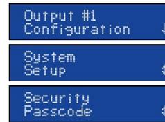
Press the Enter button to display the initial menu screen. This screen allows you to select the Output configuration, the System Setup, and the Security Passcode.
